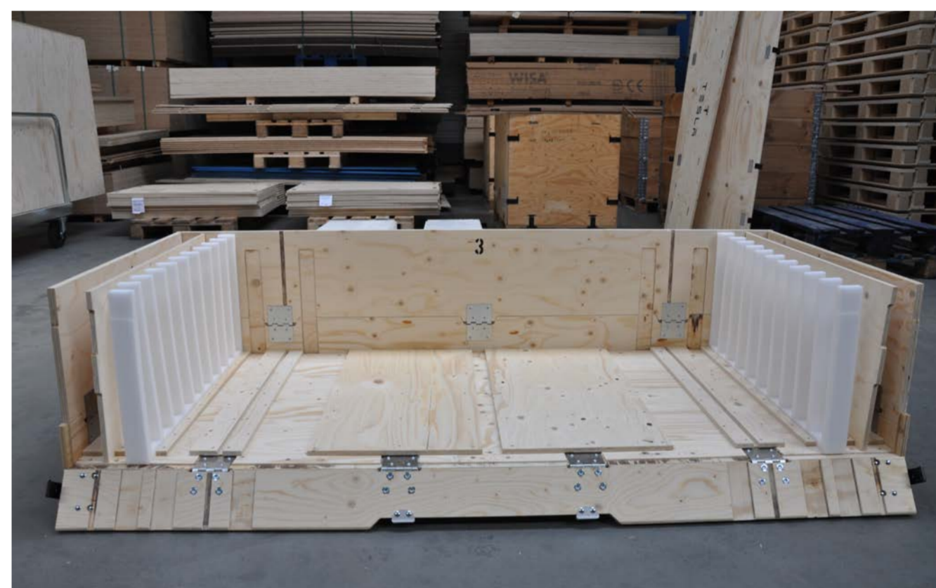
Clip-Lok 2P box built up with ETHA foam ready to protect the aluminium profiles.
