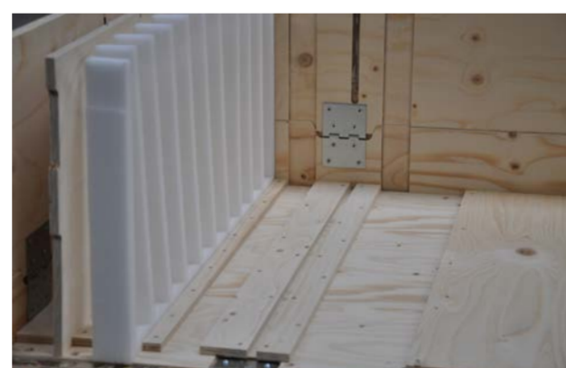
Clip-Lok 2P box flat-packed with dunnages inside the packaging.
